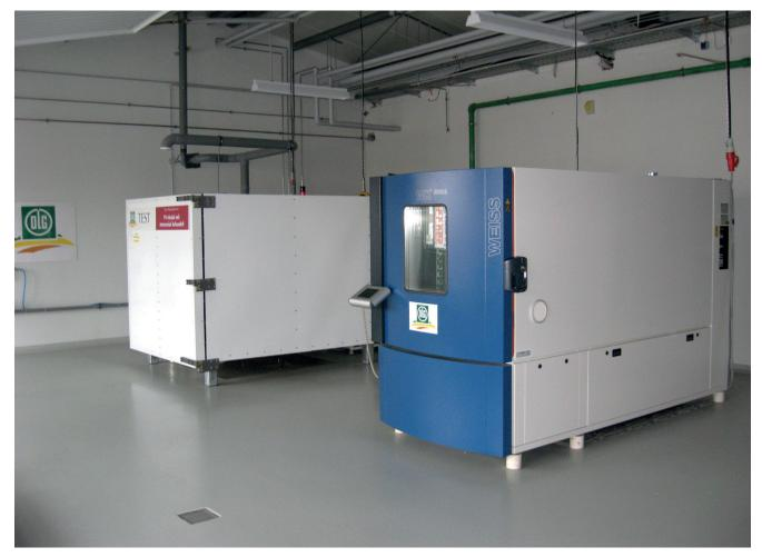
Picture 2: DLG test lab - two ammonia chambers
